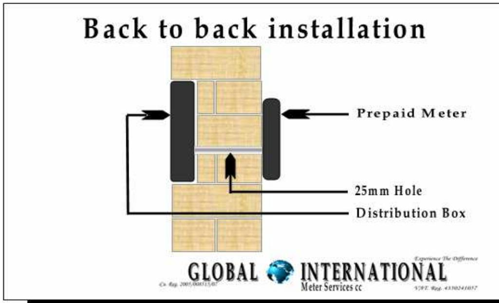
In a normal dwelling the main city council supply cable from outside feeds the distribution board inside your house / flat and is directly connected to the main circuit breaker. This main supply cable must be switched off before you re-route the cable. The life, neutral and earth wire need to be ferralled (10mm / 16mm ferrals) through / extended, therefore re-routing the main supply cable to first feed the prepaid meter and then feeding the main distribution board inside your house / flat.
